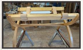
Next was the cover which the baker uses as a work surface as well as a dough cover. I acquired some hard maple from McKittrick's. After flattening and thicknessing I glued up the blank. Once the glue dried, I hand planned the surface smooth and then sanded to 150 grit. All surfaces that food would touch received a couple of coats of Mineral Oil. The stand and the bottom of the bowl were coated with Linseed Oil.
