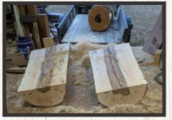
Then it was simply removing a large portion of the material in the middle. "Simply" in no way implies easy. I began with a smaller chainsaw cutting along the length of the log and the chopping the best I could to remove the waste.
