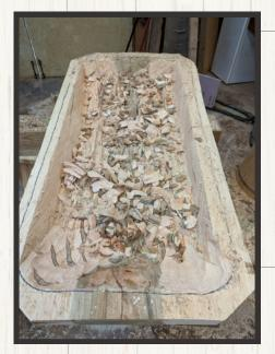
I purchased a special wood grinding attachment for my grinder and that tool aided in the clean-up of the tear outs that are inevitable when chiseling on a curve. Sanding began with 16(!) grit and ended with 150. I flipped the bowl over and cleaned up the outside and tapered the ends to a more "bowl" shape.
